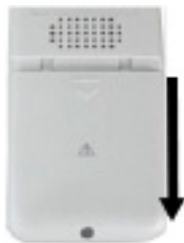
Fig 7-2 Push the battery door
