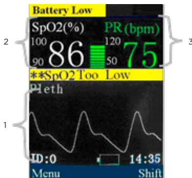
Fig 1-5 SpO 2 waveform display mode
